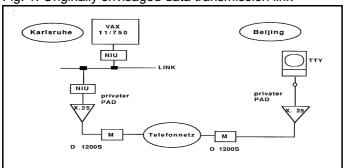
Fig. 1. Originally envisaged data transmission link
