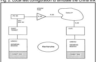
Fig. 2. Local test configuration to simulate the China link
